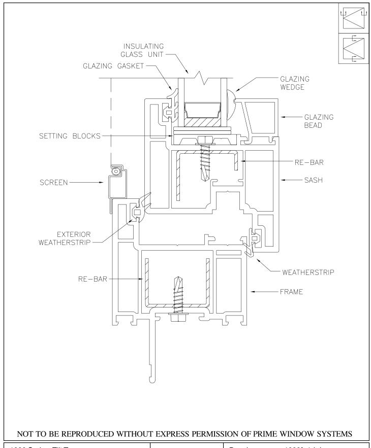
1000 Series, Tilt Turn Horizontal, Vertical Detail Scale: Full Scale
