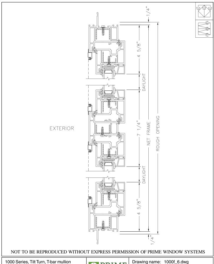
1000 Series, Tilt Turn, T-bar mullion Horizontal, Vertical Section
