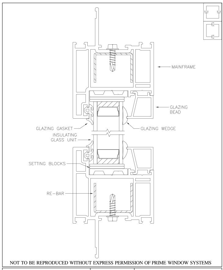
1000 Series, Tilt Turn Horizontal, Vertical Detail
