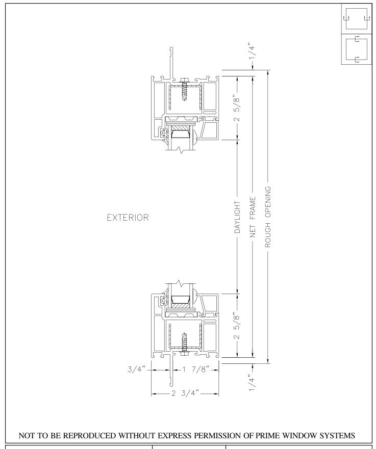
1000 Series, Tilt Turn Horizontal, Vertical Section
