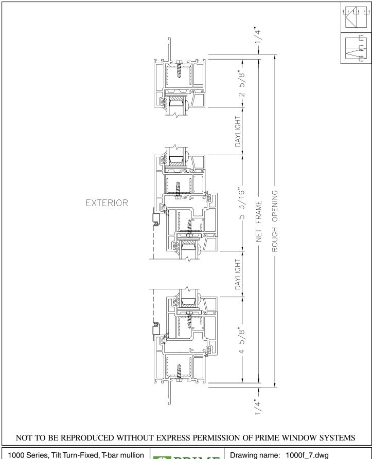
Horizontal, Vertical Section Scale: 3/8 Scale
