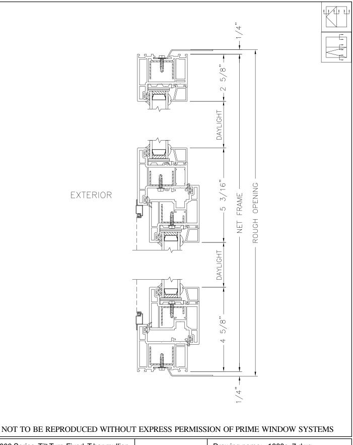
1000 Series, Tilt Turn-Fixed, T-bar mullion Horizontal, Vertical Section
