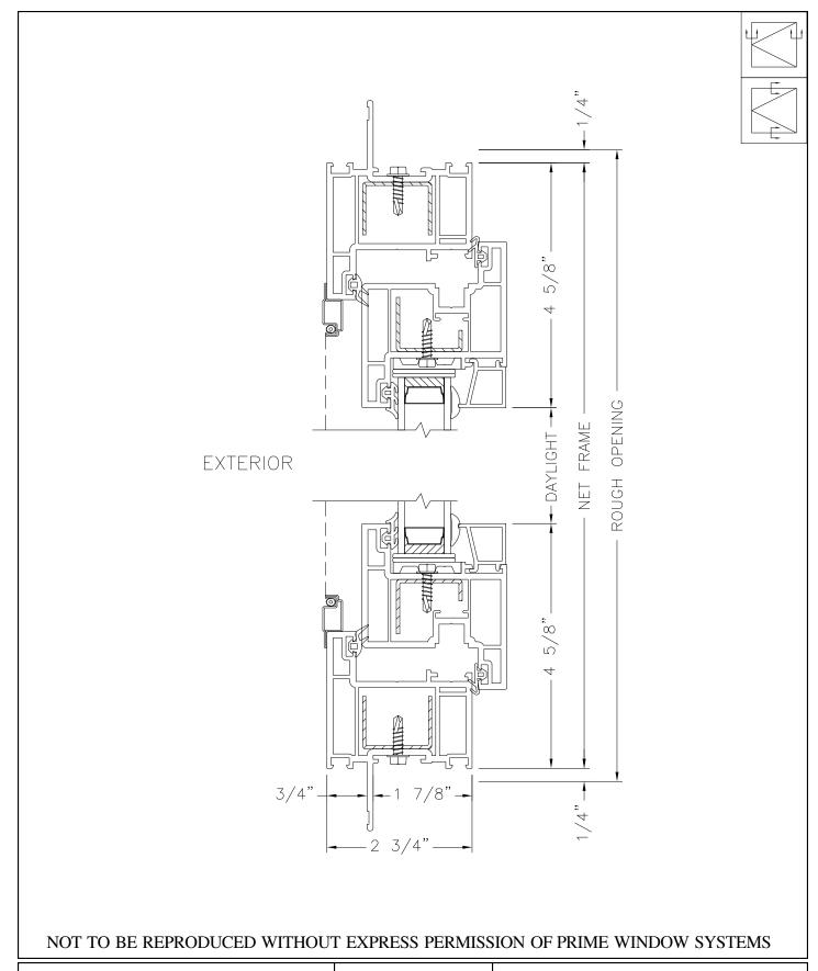
1000 Series, Tilt Turn Horizontal, Vertical Section
