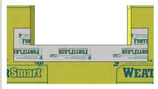
After the house wrap product has been applied, ensure the Rough opening (RO is 1/2"greater in width and height than the net frame size of the window.
