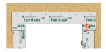
Cut the 12" SAF side flashing 16" taller than the height of the RO. Hold the flashing so that it extends into the RO 4". If the window frame is greater than 4" increase the dimension the SAF comes into the RO to match the dimension of the window frame.
