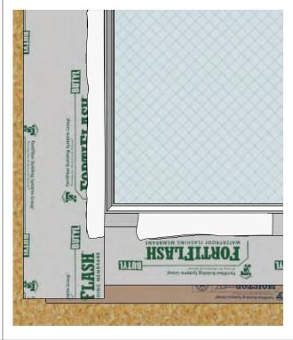
Install a 1/2" wide tubular shaped cap bead of sealant on top of the nail fins, avoiding the areas at the lower nail fin with gaps in the sealant.
