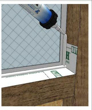
Cut top Flashing the width of the RO + 2x the dimension of the flashing plus 2". This will allow the flashing to extend 1" beyond the sideflashing on each side. Apply top SAF flashing and secure top edges with staples.
